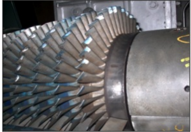
Figure 1: Compresor Axial de la Turbina a Gas
