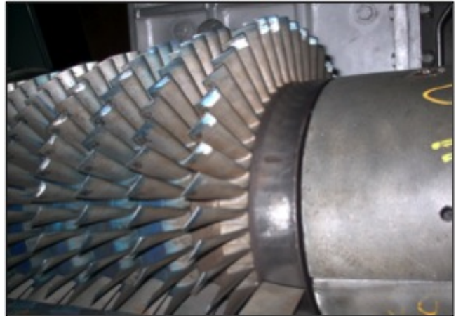
Figure 1: Axial Compressor of the Gas Turbine
